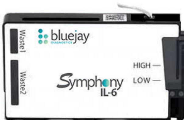
Figure X3. Photograph of the Symphony IL-6 Cartridge loaded with a whole blood specimen.
