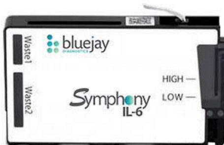
Figure 3. Photograph of the Symphony IL-6 Cartridge loaded with a whole blood specimen.
